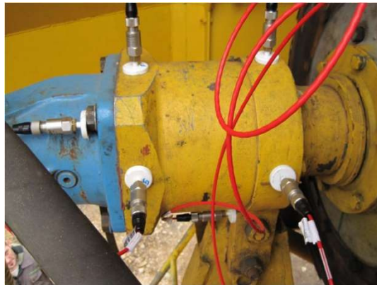
Figure 7. Sensor positions on UT reducers.
