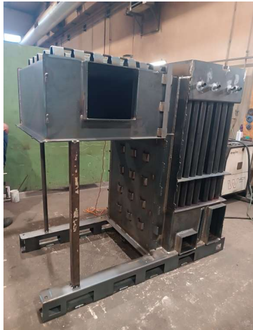
Figure 10. TX/TM boiler construction
