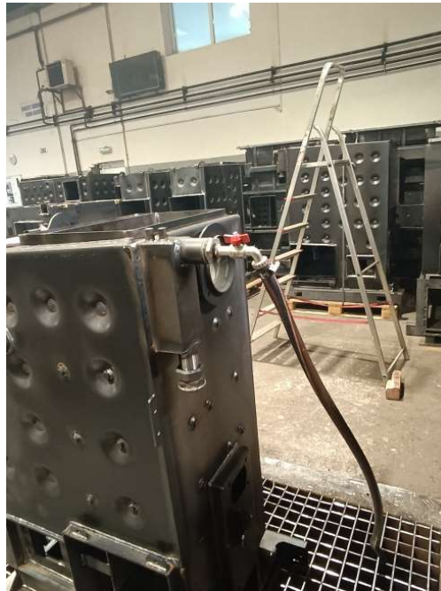
Figure 6. Connecting the valve at the highest point of the boiler to the hose
