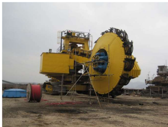
Figure 2. Rotary excavator SH 630 on the plateau where the overhaul was carried out.
