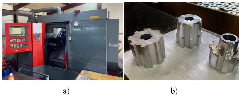
Figure 6. “EMCO” Turn465-C turning machine a) and a notched element shown in stages of machining b).
