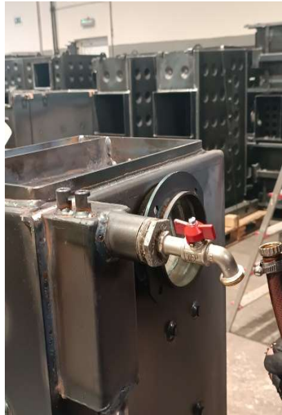
Figure 5. Valve placed at the highest point of the boiler
