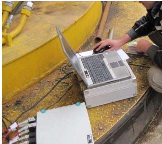
Figure 10. Appearance of used vibration measurement equipment.
