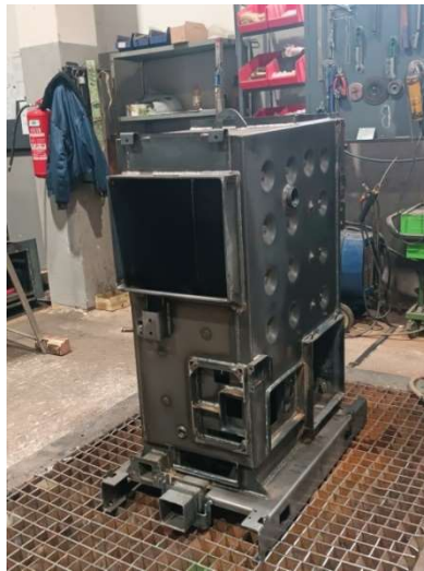
Figure 1. Welded construction of the boiler T4e 35
