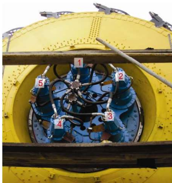
Figure 4. Layout of the impeller reducer.
