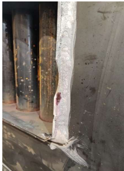
Figure 14. Detection of penetrant indications
